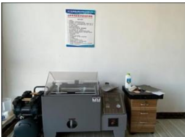
Hydrochloric Acid Corrosion Test
